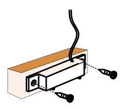
You can attach the sensor to a slightly heavier piece of wood or brick to keep the sensor in position
