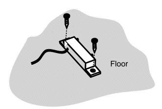
To keep the sensor fixed, you can also affix the sensor to floor by screw mounting to the floor. The metal clips can detect water as soon as water touches the clip.
