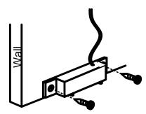
In spots closer to the wall, you can screw mount the sensor to the wall to keep it in position. You can also use a small piece of wood to screw mount the sensor to add more weight so it says at the spot you prefer.
